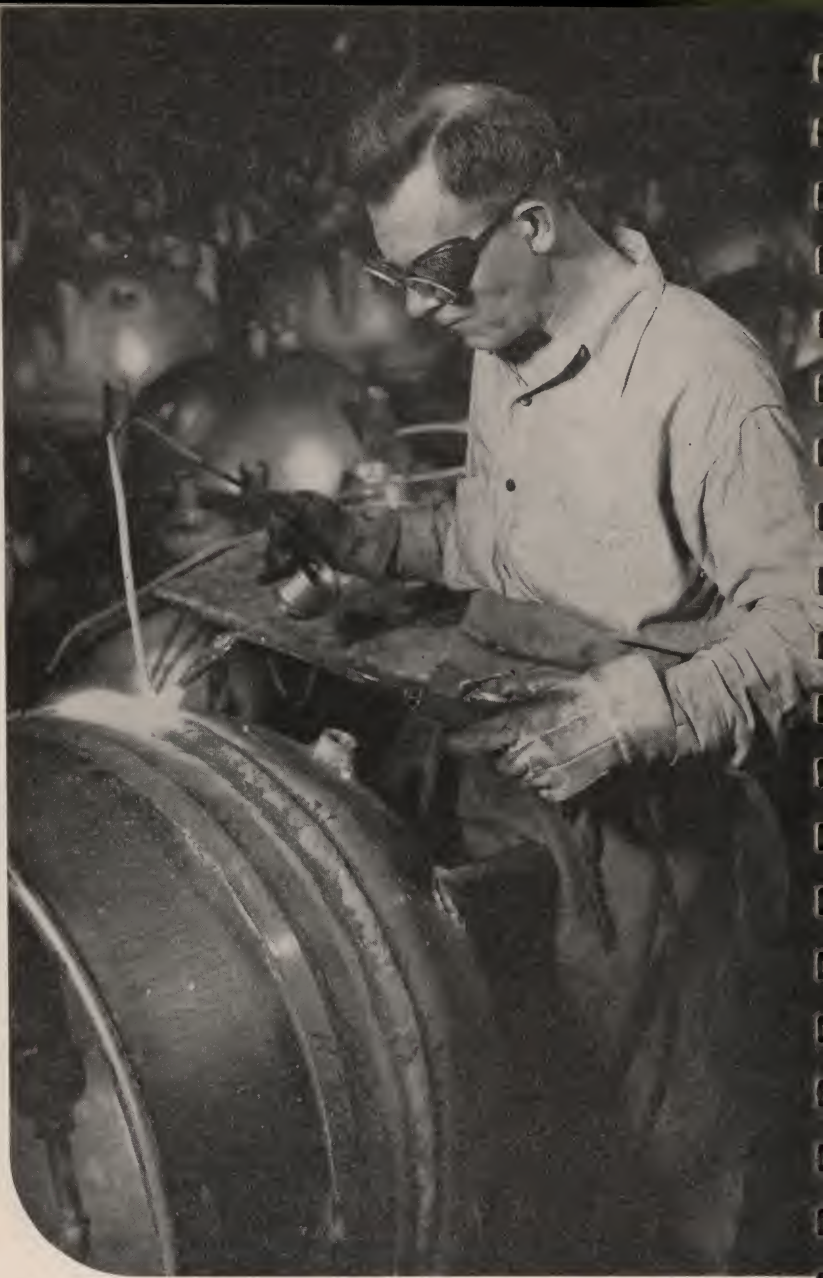
Torch welding aluminum.
